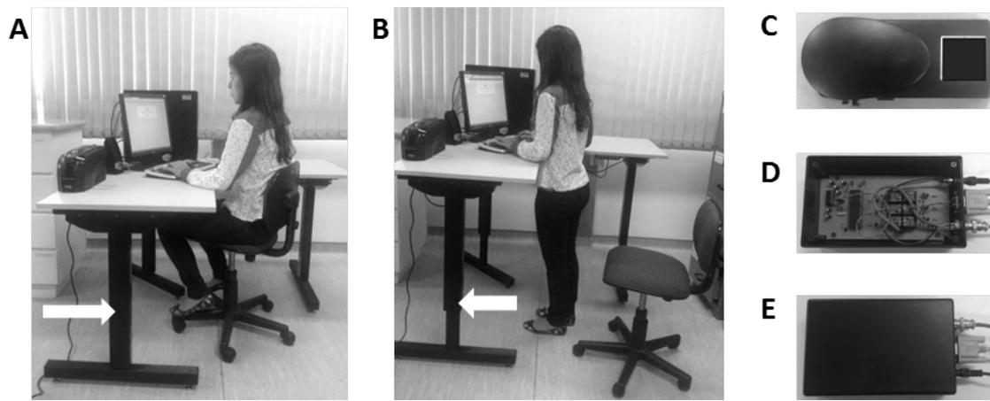
Figure 1. (A-B) Electric lifting legs (arrow) of the sit-stand table; (C) remote control for basic settings and (D-E) remote control for ongoing interaction.
