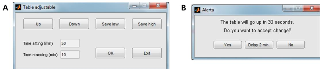
Figure 2. (A) Interface to set the reference position for both sit (low, save low) and stand (up, save high), and save the time for each position (Time sitting and Time standing); (B) Interface to warn the workers about changing the position of the table.
