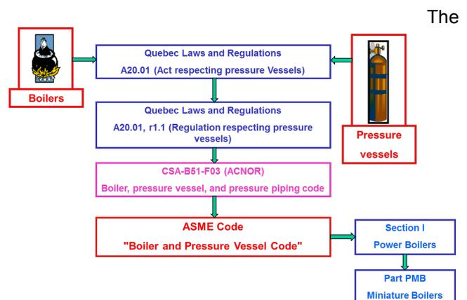
Figure 2. Applicable standards of miniature boilers
