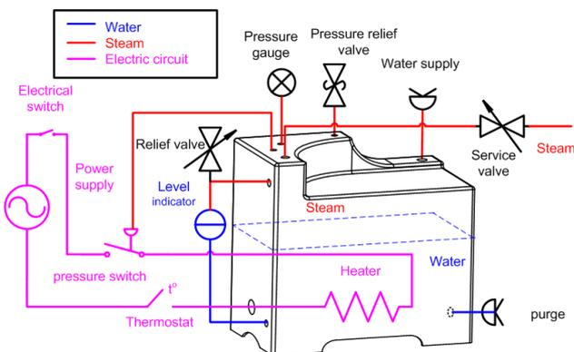
Figure 1. Steamer Machine (Miniature Boiler)
